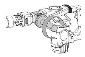
4. Check the additional handle (8) for tight fit. If necessary, tighten the additional handle further.
