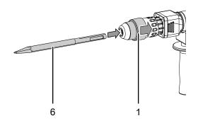
4. Check the tool for tight fit by pulling on the tool.
