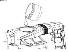
3. Put the lid (9) back on the filling hole and fasten the lid using the two-hole spanner (4).
