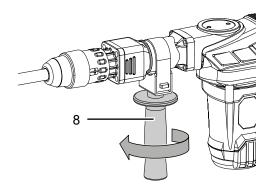
2. Turn the additional handle (8) into the desired position.
