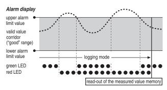
The alarm display is extinguished by reading out the measured value memory. Additionally, a hysteresis can be set, by which value the measured value must re-enter the valid range in order to switch off the alarm.
