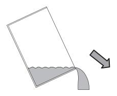
3. Rinse the condensation tank with clear water. Regularly clean the condensation tank using a mild cleaning agent (no detergent!).
