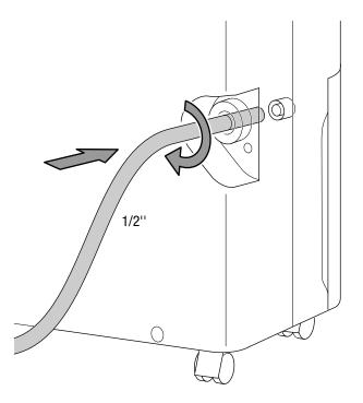
Guide the other hose end to a suitable drain or sufficiently dimensioned collection container. Please note that the hose must not be kinked.
