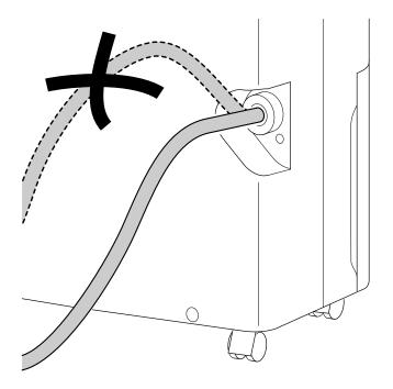
Remove the hose if you want to collect the condensate in the condensation tank again. Allow the hose to dry prior to storage. The hose can be connected in any operating mode for continuous operation.
