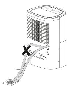
Remove the hose if you want to collect the condensate in the condensation tank again. Allow the hose to dry prior to storage.
