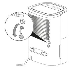
2. Push one end of the hose onto the hose connection.
