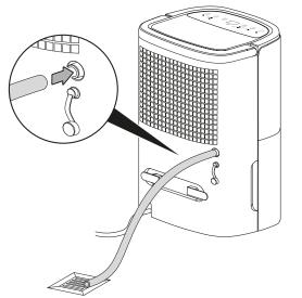
3. Guide the other hose end to a suitable drain or sufficiently dimensioned collection container. Please note that the hose must not be kinked.
